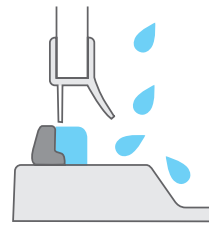
Threshold strip at the bottom of the shower enclosure: Brilliant, SmartLine, Matrix, Chrome
